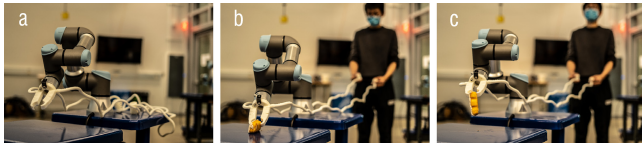
Figure 20: The printed robotic gripper: a) the printed assembly is installed to an UR3 robotic arm; b) the gripper aims for the cake; c) the gripper is activated to lift the cake with the operator at a distance.
