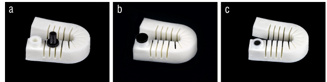
Figure 9: a) Printed parts with a drain hole and a drain plug; b) the assembled drain hole; c) the cross section of the plugged hole.
